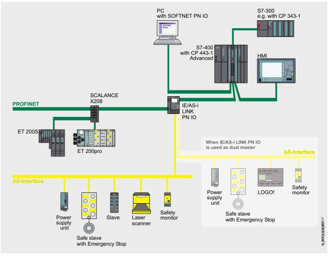
Linking of AS-Interface to PROFINET via IE/AS-i LINK PN IO as single/dual master
