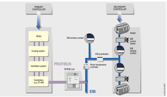
DP/EIB Link as a link for HVAC systems (heating, lighting, air conditioning) between the primary and secondary control systems
