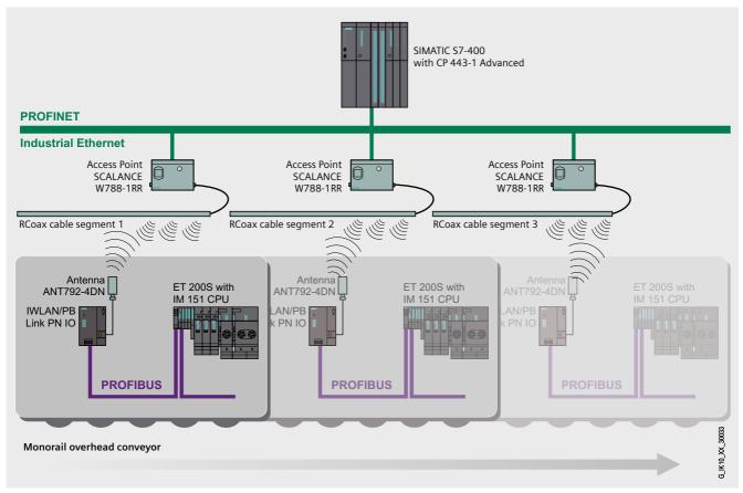
System solution with IWLAN/PB Link PN IO using example of monorail overhead conveyor
