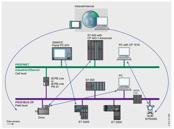
Sample configuration of IE/PB Link as network transition from Industrial Ethernet to PROFIBUS for vertical integration
