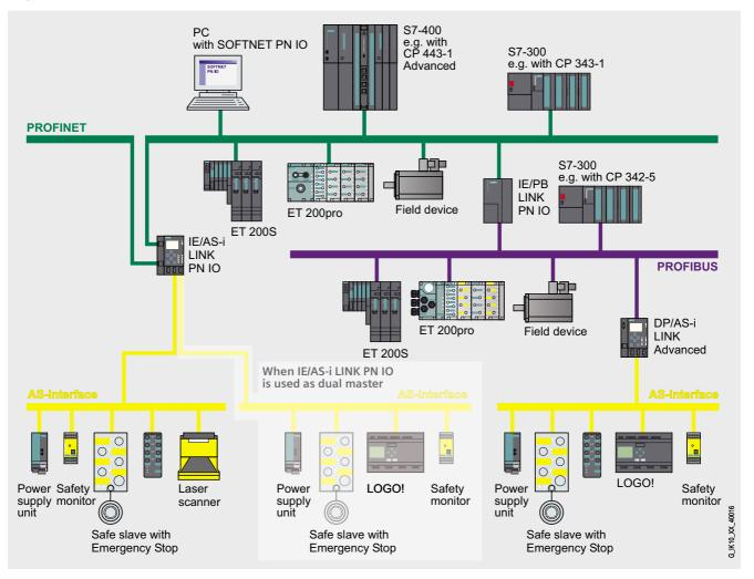
Network transitions from one bus system to another are implemented using links, PLCs or PCs. In the case of PLCs or PCs, this can take place via integrated interfaces and communications processors (CPs). Links pass on the data autonomously from one network to the other.
