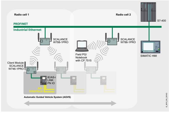
Wireless communication between Industrial Ethernet and AS-Interface components
