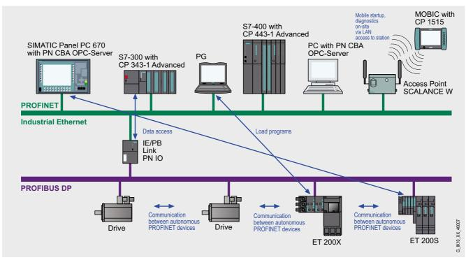
Sample configuration of PROFINET with Industrial Ethernet and PROFIBUS. Over the IE/PB Link as proxy, PROFIBUS devices can be seamlessly incorporated in the PROFINET.
