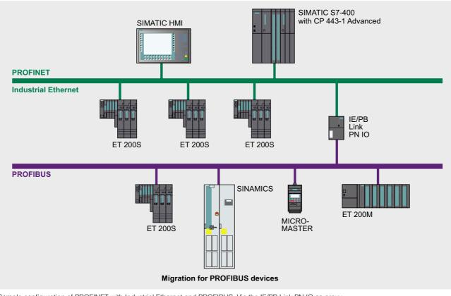
Sample configuration of PROFINET with Industrial Ethernet and PROFIBUS. Via the IE/PB Link PN IO as proxy, PROFIBUS devices can be seamlessly incorporated in the PROFINET.
