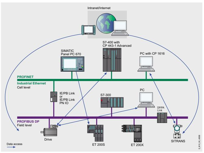
Sample configuration of IE/PB Link PN IO as router from Industrial Ethernet to PROFIBUS for vertical integration
