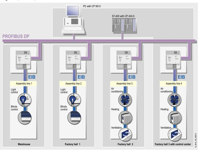
Connection of EIB applications to a PROFIBUS network that spans buildings
